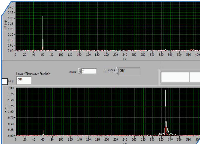
Figure 9. Frequency Responses of the Strain Gauges in the Six-inch Pipe at 108.1 ft/s
